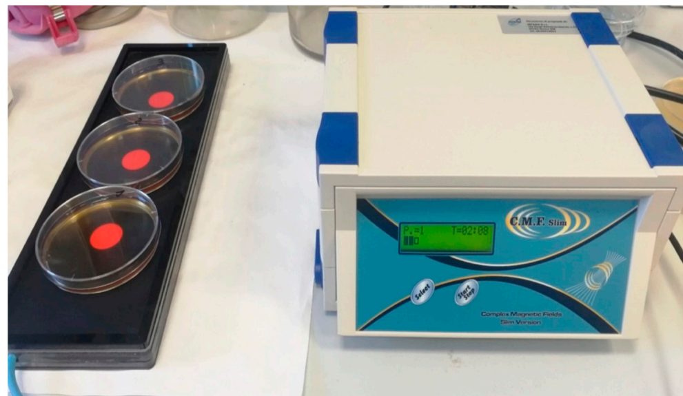
Figure 1. Culture samples of Candida albicans ATCC 10,231 during the treatment with complex magnetic fields (C.M.F.s).
