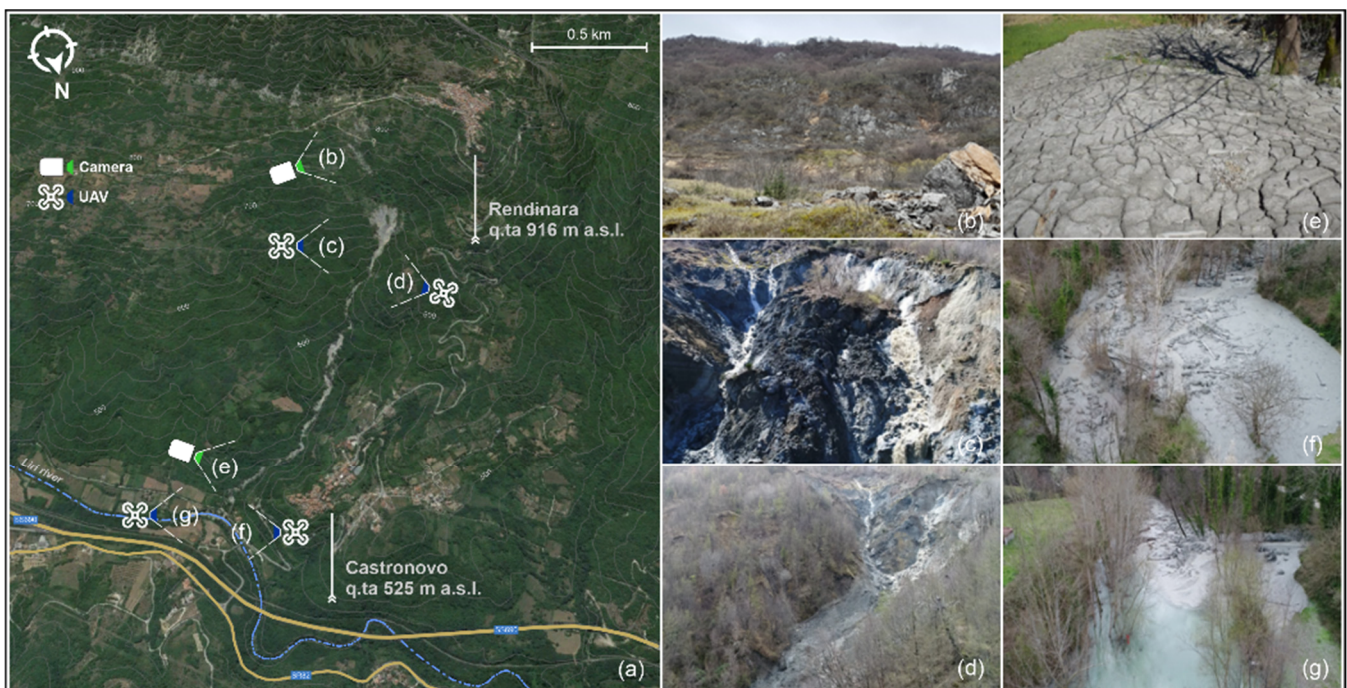
Figure 1. Aerial and field images of the Morino-Rendinara landslide that are representative of the impact of the landslide on the environment. (a) Overview of phenomenon taken from Google Earth [16] satellite images of 13 June 2022, from the upper sector near Morino Hamlet to the lower sector, Liri River, and deep-seated rotational slide; (b) Details of rockfall/avalanches sector; (c) Debris flow source area; (d) Debris flow transit zone; (e) Lowest debris flow transit zone; (f) Liri River dam; and (g) Effect on Liri River dam.
