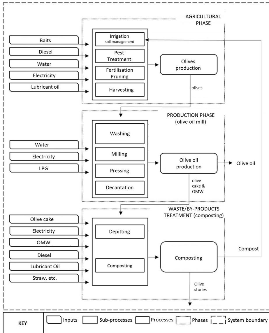
Figure 4. Flow Chart for the Olive Oil product system
