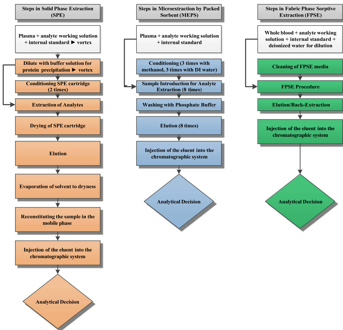
Fig. 3. Schematic representation of the steps involved in SPE, MEPS and FPSE.
