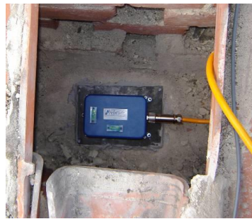
Figure 13 – Dynamic monitoring system [7]: (a) sensors location; (b) accelerometer A2 at the roof level; (c) battery of recorders and accelerometer A1 at the base level.
