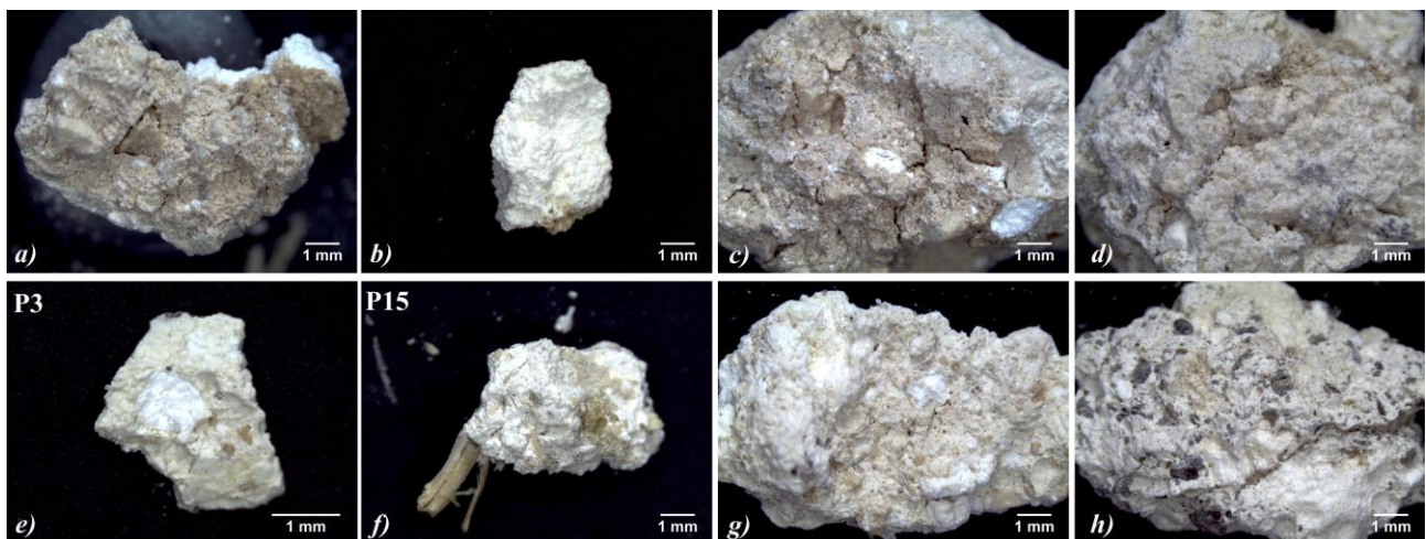
Figure 2. Stereomicroscope images of the arriccio samples taken from the following pictorial scenes: a-b ) the Dormition of the Virgin (from P18 sampling area), DV ; c ) the Saints, S (from P17 sampling area); d ) the Virgin with Child Jesus, VJ (from P25 sampling area). In b ) an isolated lime lump from DV is shown. Stereomicroscope images of the fragments of the preparatory layers taken from the following pictorial scenes: e-f ) the Dormition of the Virgin, DV ; g ) the Saints, S ; h ) the Virgin with Child Jesus ( VJ ).
