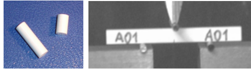
(b) Example of the specimen (c) Three bending point test of the specimen
