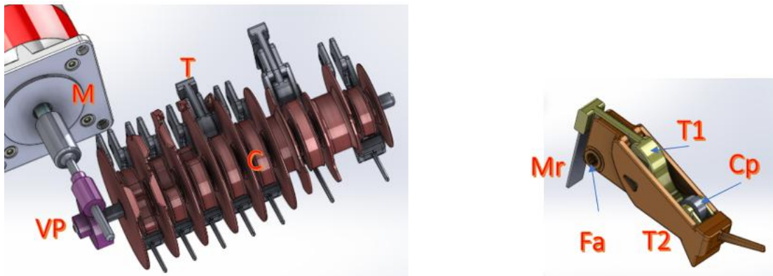
Figure 9. Details of the Valve System and Buttons.
