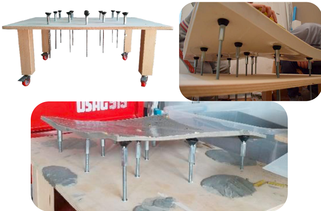
Figure 8 Prototype machine for the production of the double-curved shell with the pin pad system (left), mould (right) and concrete casting (bottom).
