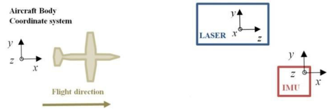
Figure-2. Aircraft body coordinate system (left) and reference axes of the laser and IMU in bottom view (right).
