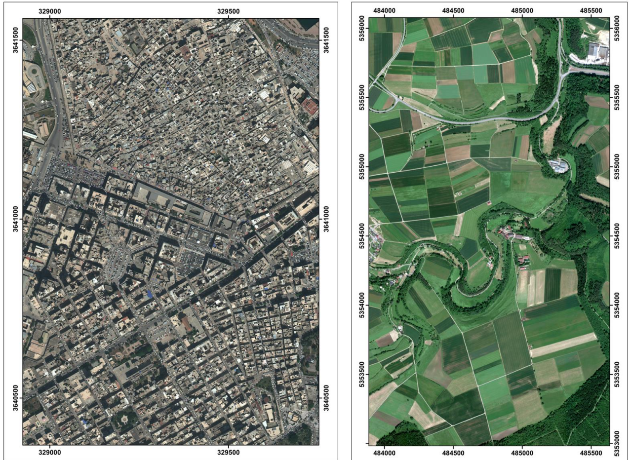
Fig. 4: Multispectral LRMS Scene of Worldview3 in RGB (5-3-2 Composite Bands): (Left Image) Urban Area (Libya) - Projection: Transverse Mercator; WGS 1984 UTM Zone 33N; (Right Image) Rural Area (Germany) - Projection: Transverse Mercator; WGS 1984 UTM Zone 32N.
