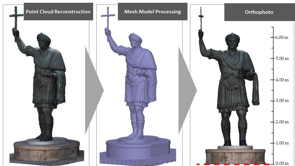
Figure 4. Three-dimensional models view and orthophoto generated by the photogrammetric process.
