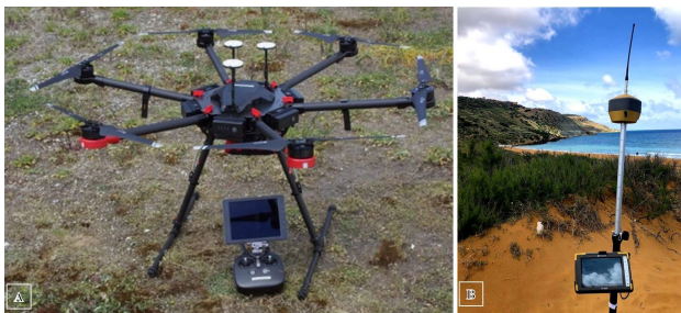
Figure 2. Example of AUV used for acquisition of the data Matrix 600 (a) and the Topcon Hyper HR Base-Rover satellite acquisition system used for GCPs data acquisition (B).
