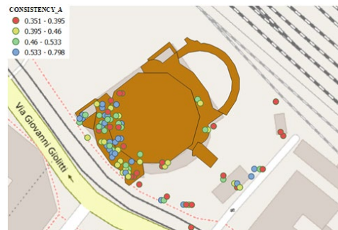
Figure 5. Distribution of monitored points as the consistency variation relating to the ascending orbit [QGis3.10 A Coruña]
