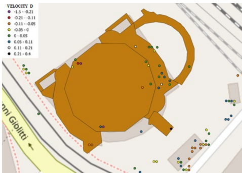
Figure 4. Spatial distribution of annual velocity values (cm/year) relating to the descending orbit [QGis3.10 A Coruña]
