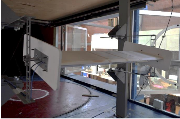
(a) View of pressure tests at CRIACIV Boundary Layer Wind Tunnel lab.
