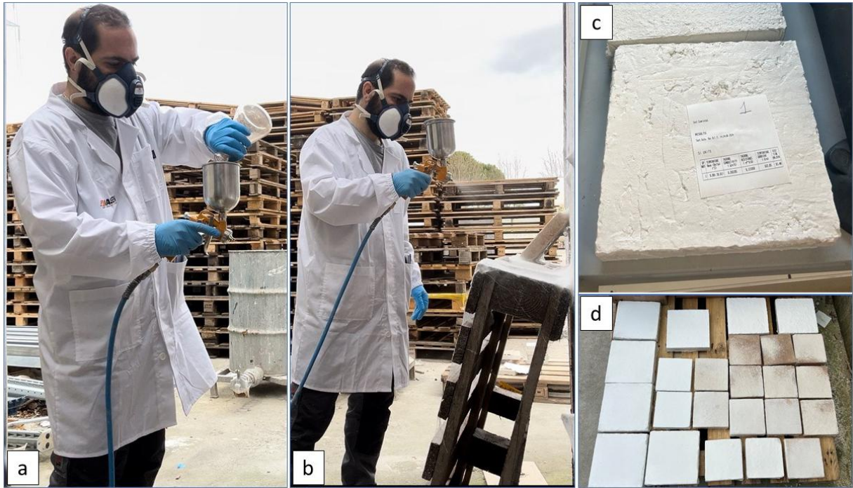
Figure 39. Spray coating process at Diasen Company. a) Pouring the slurry composite into the coating spray tank, b) applying of the slurry composite (using the air pressure), c) concrete specimen with measured baseline thermal conductivity, ready for coating, and d) freshly coated specimens, still wet.
