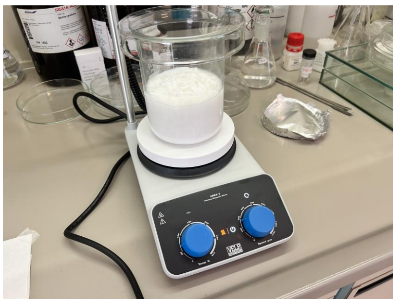
Figure 32. The slurry production process under the magnetic stirring at elevated temperatures
