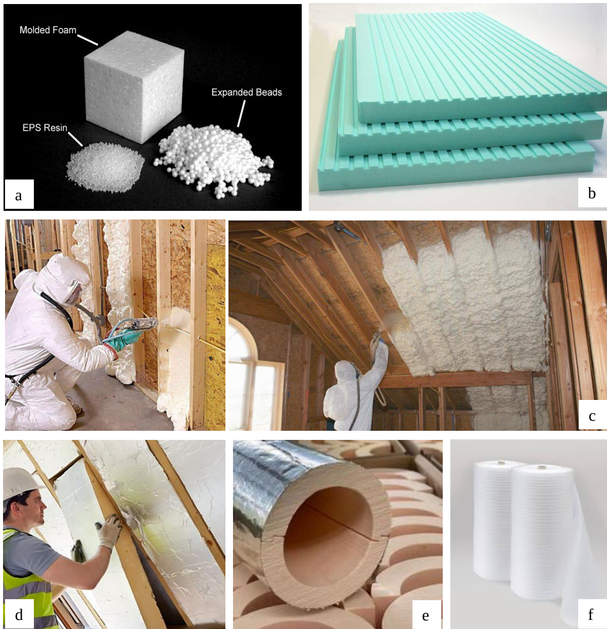
Figure 9. Organic insulation material (Petrochemical-based) a) Expandable polystyrene (EPS), b) Extruded polystyrene (XPS), c) Polyurethane (PU), d) Polyisocyanurate (PIR), e) Phenolic Foam (PF) and f) Polyethylene Foam (PEF)
