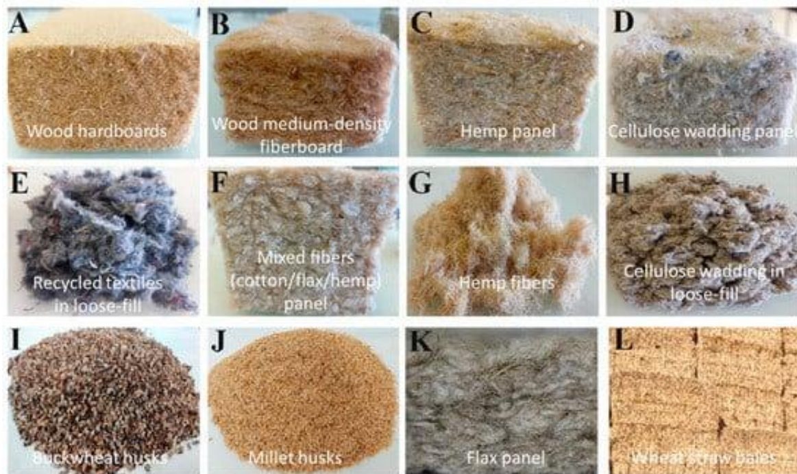
Figure 15. Various bio-mass-based sustainable materials for thermal insulation; (A) wood hardboards; (B) medium density wooden fiberboard; (C) Hemp panel; (D) Cellulose panels in compacted form; (E) recycled textile fibers; (F) mixture of cotton, flax and hemp fibers; (G) hemp fibers; (H) cellulose fiber in loose fill; (I) wheat husk; (J) millet husk; (K) flax panel; and (L)wheat straw bales [126].
