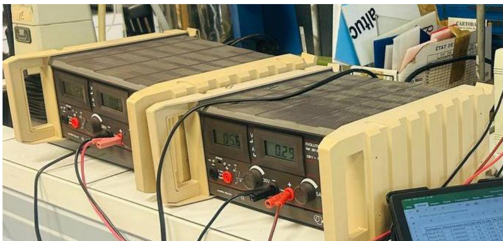
Figure 47. The power alimentations used for hot disk thermal analyzer
