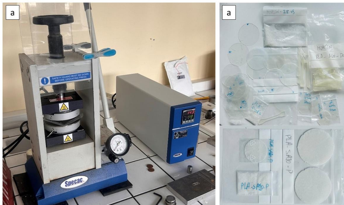
Figure 42. a) The Specac Atlas™ Manual 15T Hydraulic hot presses used to produce film specimen, and b) The film samples made by the Hydraulic hot presses
