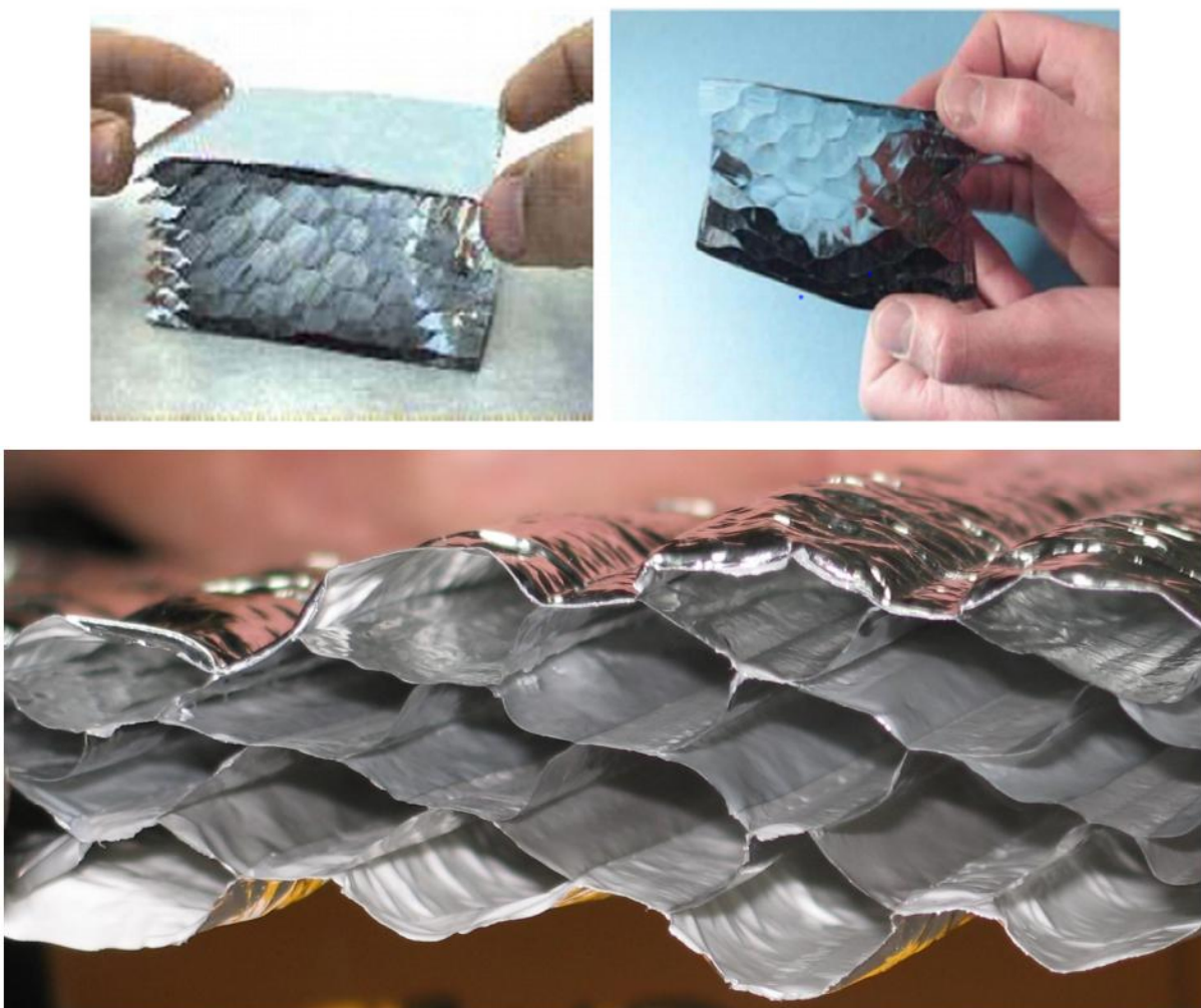
Figure 26. An inside view of GFP on the barrier foil with baffle structure (up) [136] and Honeycomb structure of the GFP by cutting one panel.
