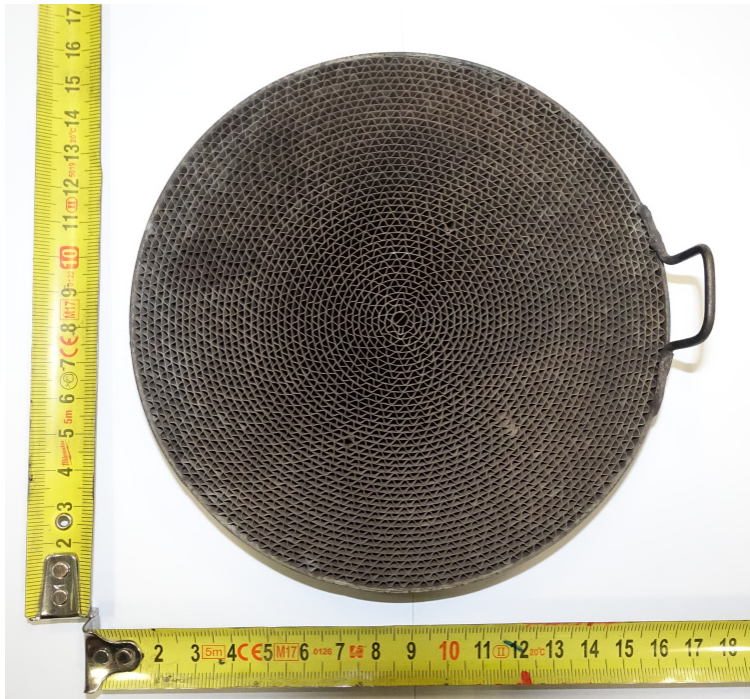
Figure 1: Honeycomb catalyst before combustion tests.
