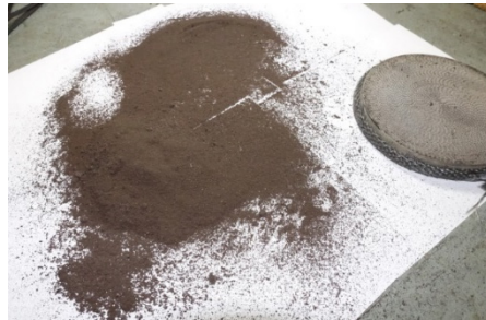
Figure 4: Cleaned catalysts with the removed particulate matter after Stove 1 tests.
