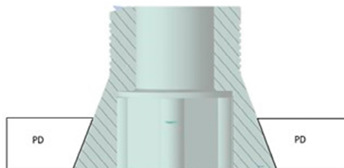
Figure 6. Cone–Morse connection at the screw–PD interface.
