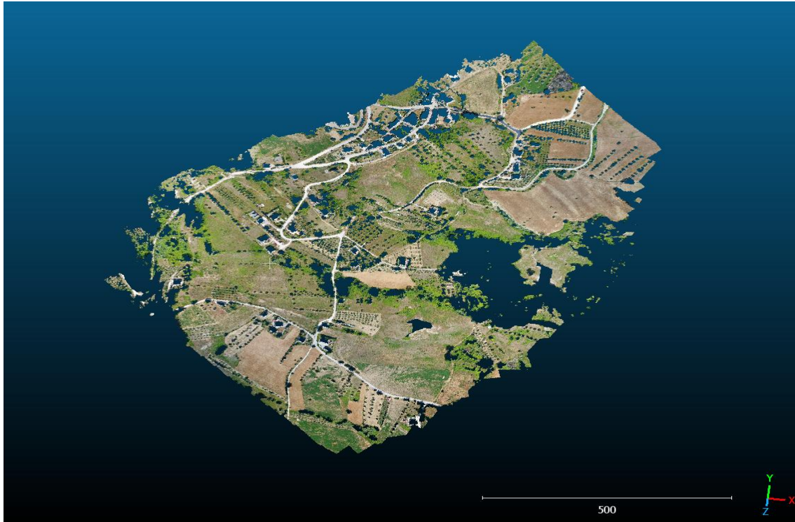
Figure 13 DEM data from drone surveyed data after editing data in CloudCompare software [44]
