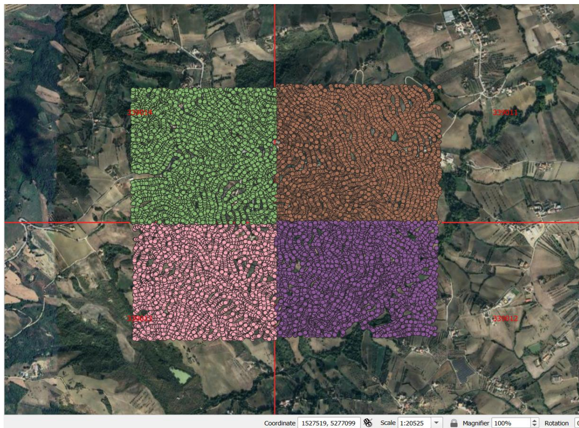
Figure 8 Extracting vertices contours SHP data into point data including z coordinates through QGIS software for the total of the study region [40]
