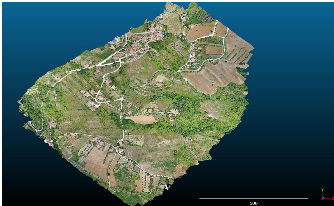
Figure 12 DEM data from drone surveyed data before editing points in CloudCompare software [44]
