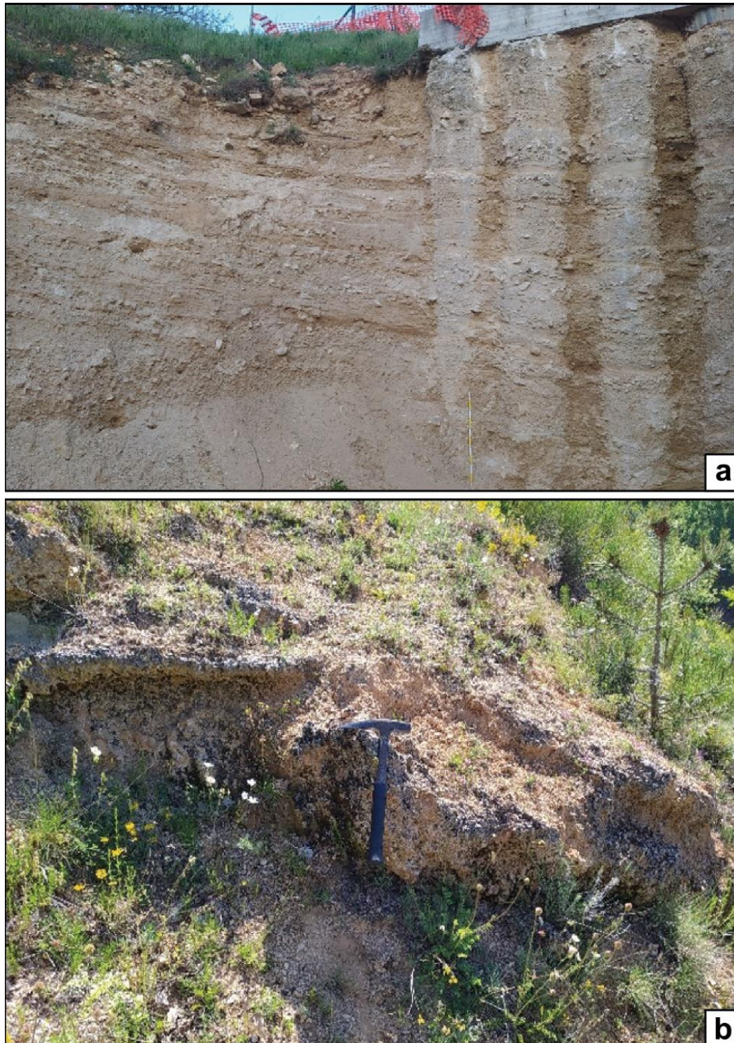
Figure 4.8. a) Stratified sandy gravels with heterometric clasts with millimeter to decimeter size, subrounded to subangular, in silty-sandy matrix, alternating with silty-sandy levels. Outcrop in a recent man-made excavation in the Frattale locality (Pizzoli, AQ) at one of the fault segments. These are referable to unit 3 of the main map. b) Heterometric angular breccias with millimeter to centimeter clast size, clast-supported, sandy-loam matrix, well cemented suspended in slope support at the fault bed east of the Villa Mazza quarry (Pizzoli, AQ). These are referable to unit 2 of the main map.
