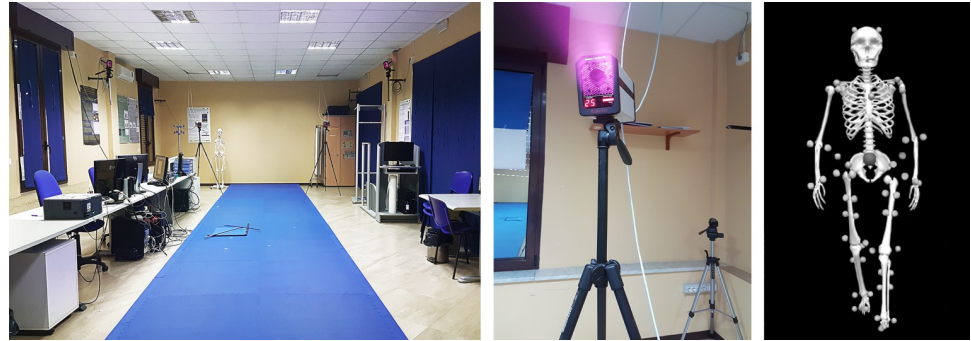
Fig 1. Acquisition setup. The left panel shows the acquisition setup. The centre panel shows details of one of the eight cameras employed for the acquisition. The right panel shows a representative image of the patient's acquired data.
