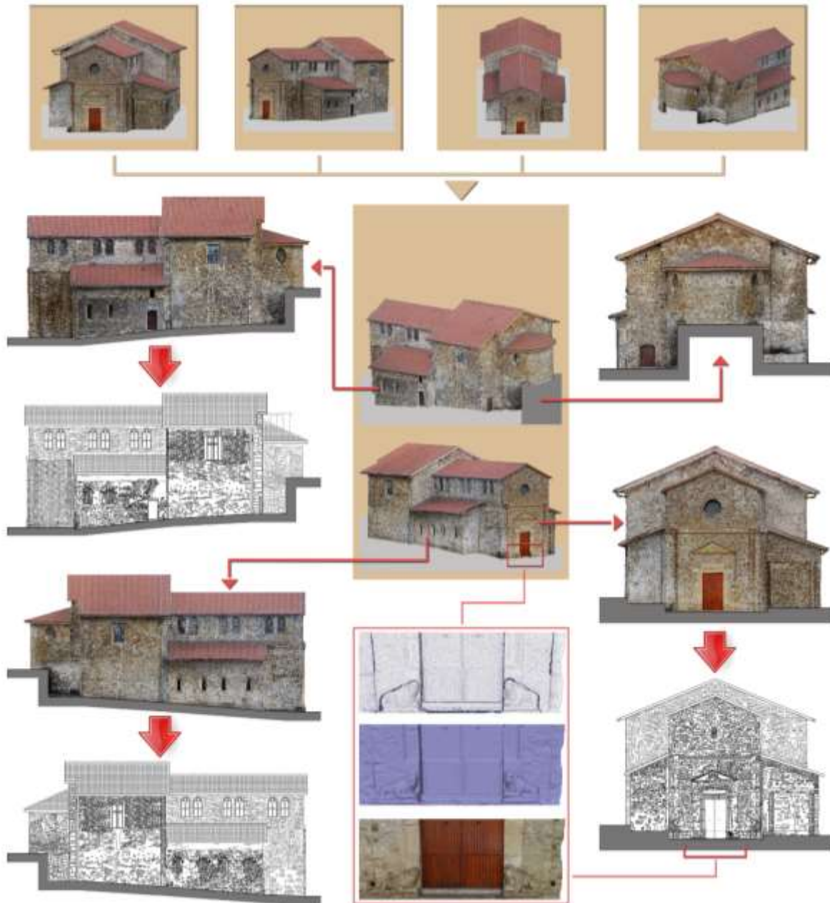
Figure 5 Metric survey of the church: from 3D to 2D representation
