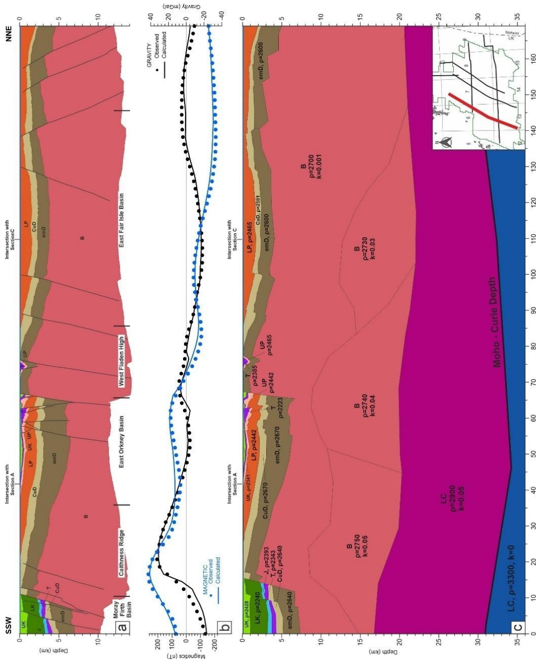
Fig. S2.2 Gravity and magnetic anomalies model across the Section D (seismic line name: OA16ESP00039A032). (a) Depth-converted section. (b) Anomaly curves best fitting. (c) 2D
