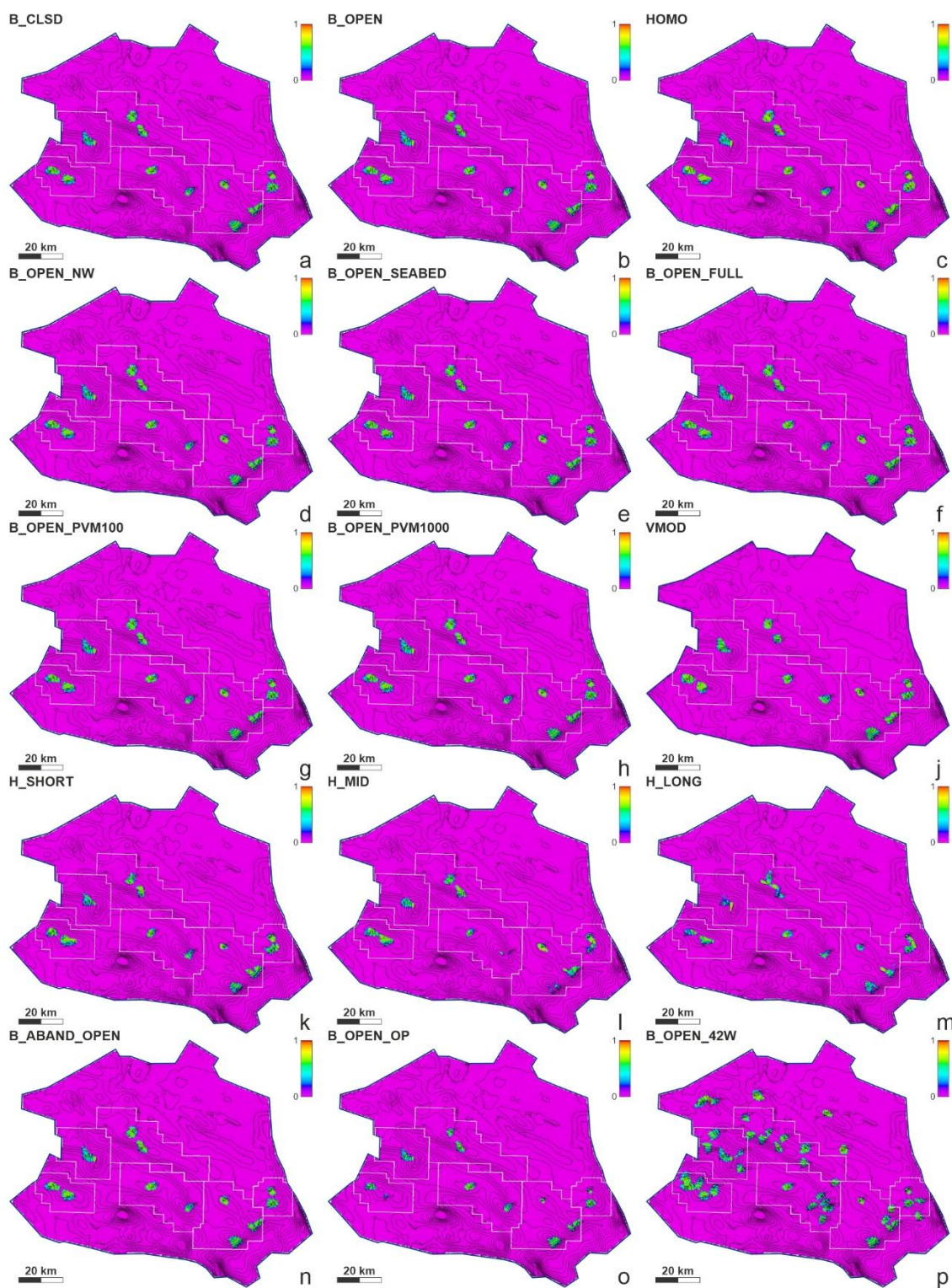
Fig. S3.10 CO 2 saturation 100 years after Cessation of Injection (COI).
