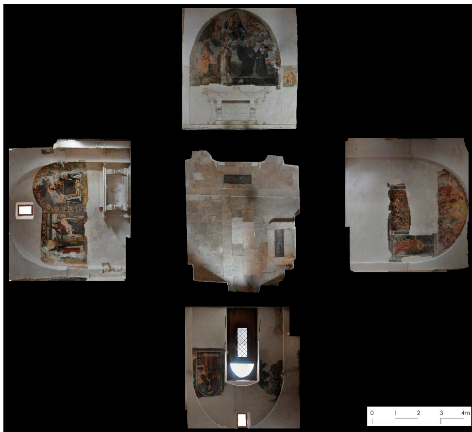
Figure 6. Orthogonal projection of the inside of the structure: orthophotos (in very high resolution) of the single façade and floor of the church.
