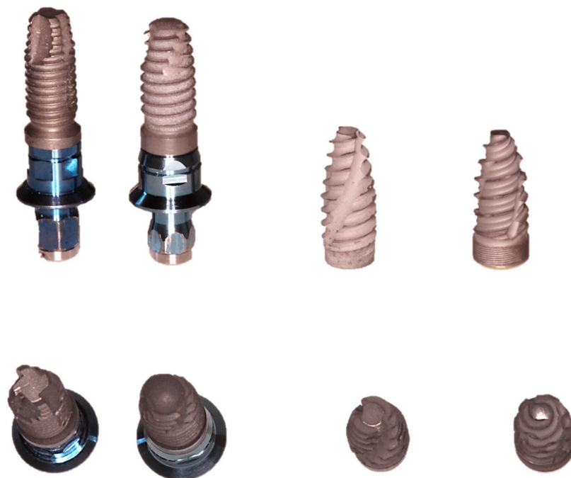
Figure 5. Different designs (lateral and top views) of the four implants used in the present in vitro study. From the left: EE, T3, TAC, and Intra-lock implants.
