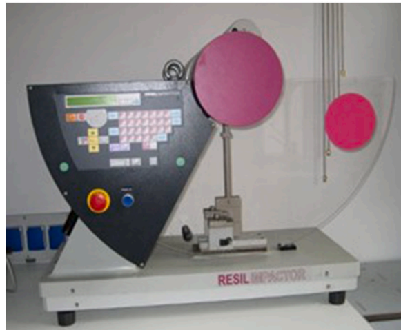
Fig. 4. Resilience test system.
