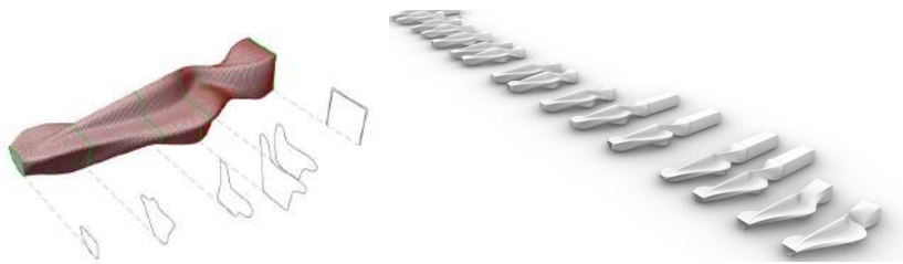
Fig. 6 Parametric design used for surface generation (Left); Exploration of different designs by means of parametric design (Right) (Courtesy of DONE Lab - Advanced Manufacturing of Products and Tools, Guimarães, Portugal).
