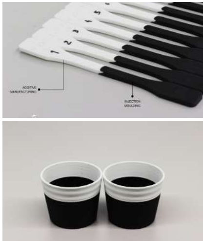
Fig. 4 Specimens produced for test analysis (left); Cup produced by FDM with ASATM overmoulded with PP (right) (Courtesy of DONE Lab - Advanced Manufacturing of Products and Tools, Guimarães, Portugal).
