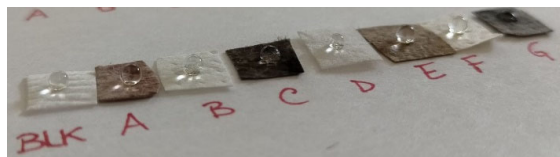
Figure 4. Contact angle of the FM samples, from the left to the right: sample Blk, sample A, sample B, sample C, sample D, sample E, sample F, sample G.
