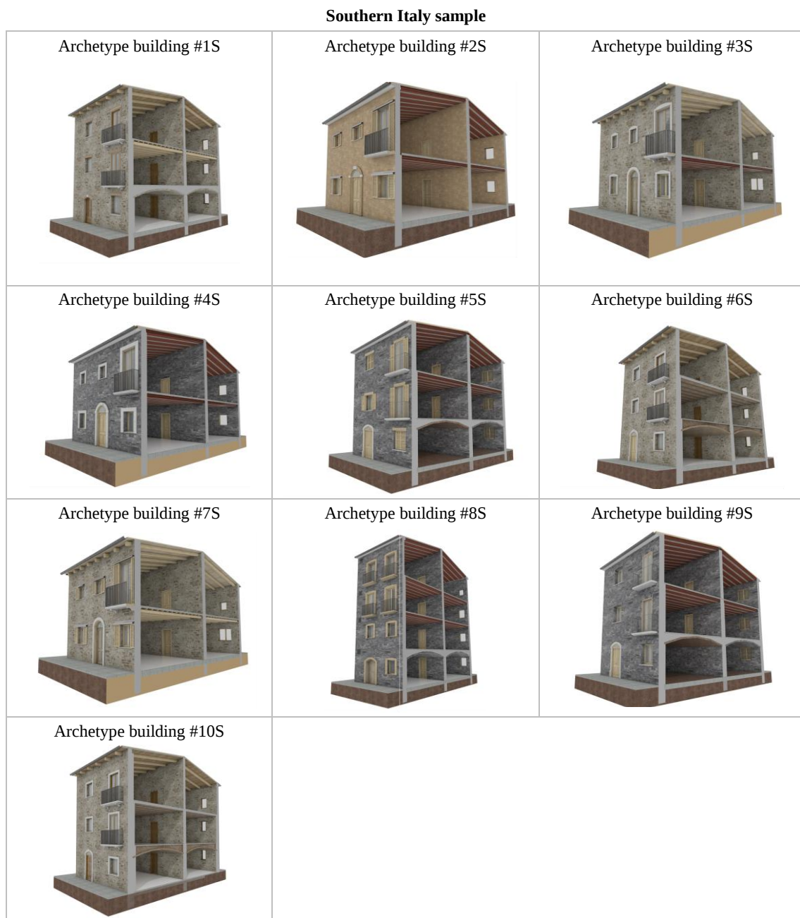
Figure 3. Graphic representation of archetype buildings for the macro-area of Southern Italy.
