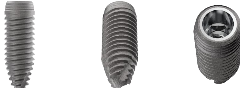
Figure 3. Details of standard-length implants tested in the present investigation. From the left: lateral, bottom (apex), and top (connection) views.
