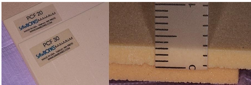
Figure 4. Details of the different polyurethane laminas of 20 and 30 PCF density used in the in vitro simulation. Right image, a 3 mm thick lamina.
