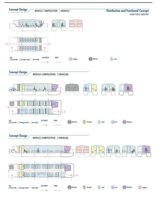
Figure 3: Modular design, platforms, and possible configurations (Cipressi, 2022).
