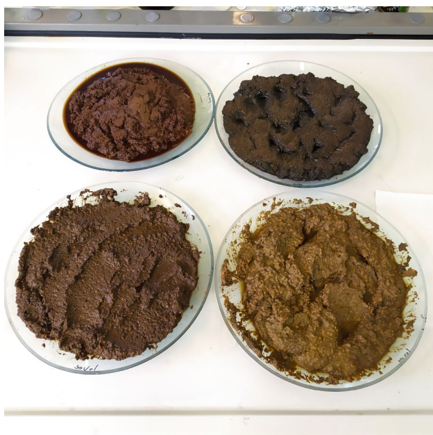
Fig. 1 Example of OP samples (WOP) untreated (top, left) and treated samples (only with Fe, on the top, on the right side; with Fe and 4.4 M H 2 O 2 , on the bottom, on the left side; with Fe and 8.9 M H 2 O 2 , on the bottom, on the right side). Note the slight whitening observed on the treated sample with the higher concentration of H 2 O 2
