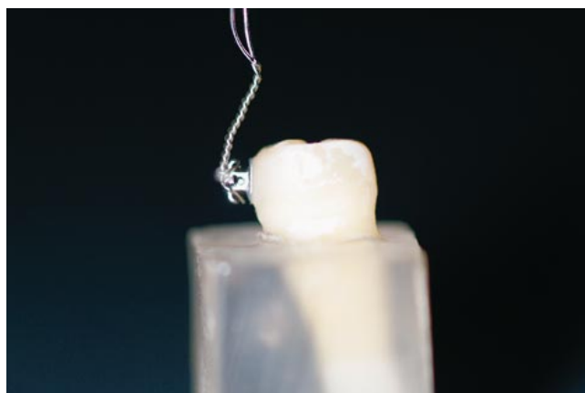
FIGURE 1. Bonded teeth set in acrylic block; a 0.021 × 0.025-inch stainless steel wire was ligated into each bracket slot to minimize deformation of bracket during debonding; a 0.020-inch loop was made from a 0.012-inch stainless steel ligature wire and placed under the gingival wings of the twin bracket.
