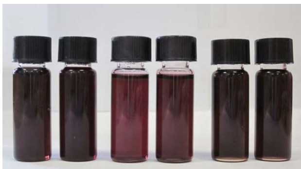
Figure 3. Samples of gold nanoparticles prepared with LD-LA (right), LA (center), DA-LA (left). For each couple the concentration of the drug/codrug is 1.0 mM in the left vial and 2.0 mM in the right vial.
