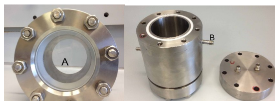
Figure 1 High-pressure reactor. A: quartz window; B: cooling jacket.
