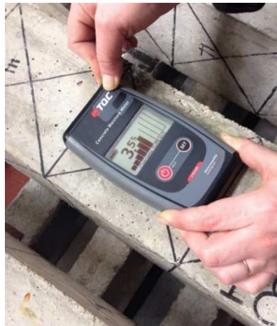
Figure 1: Measurement of impedance humidity with moisture meter
