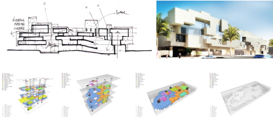
Fig. 1, Space Planning with synthetic user experience by Christian Derix, AEDAS: Abu Dhabi Education Council competition, Abu Dhabi, UAE (2009). From left to right: Initial random placement of accommodation units; interactive semiautomatic ordered layout; block model visualization; second skin for final envelope extends. (Courtesy of Aedas Architects, Christian Derix, 2014.)
