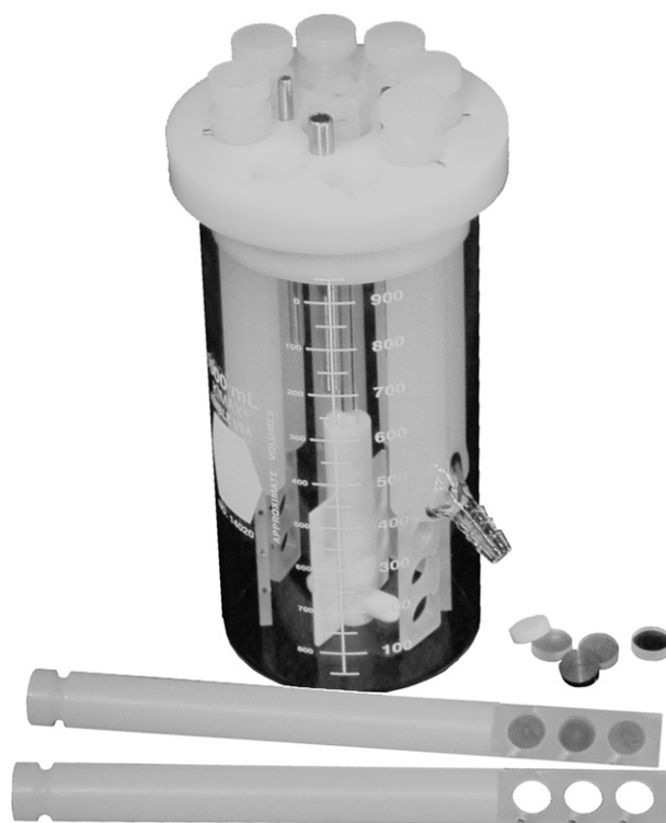
Figure 6. The Center for Disease Control (CDC) biofilm reactor. The CDC Biofilm Reactor consists of eight (8) polypropylene coupon holders suspended from a UHMW-polyethylene ported lid. The coupon holders can accommodate three 1/2 inch (12.7 mm) diameter coupons each. The lid with coupon holders and coupons is mounted in a 1L glass vessel with side-arm discharge port. A liquid growth media is circulated through the vessel while mixing and shear is generated by a magnetic stir bar rotated by a magnetic stir plate. Image and description text courtesy of Bryan Warwood, BioSurface Technologies Corp, Bozeman, MT. © Bryan Warwood. Reuse not permitted.
