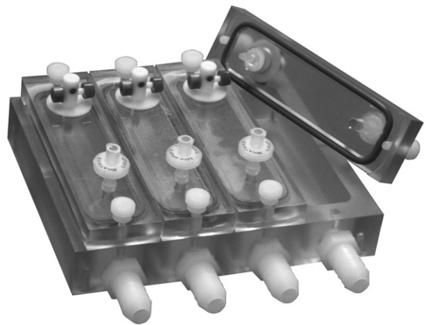
Figure 5. The Drip Flow Biofilm Reactor. Commercial version of the drip flow biofilm reactor, with four chambers each accommodating a microscope slide. © Bryan Warwood. Reuse not permitted.
