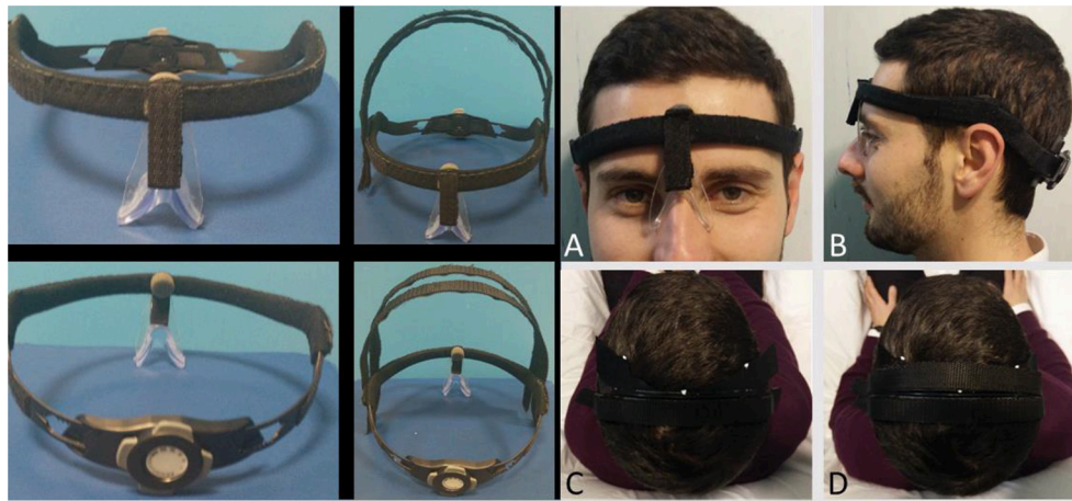
FIGURE 3 | AHF for multisession RePE repositioning. Left: Adaptable Helmet Frame (AHF) without (left) and with (right) the Velcro strips to fix RePE. The occipital cathode electrode is fixed under the adjustable mechanism. Right: As detailed in the Methods, steps (A,B) allow positioning and re-positioning the AHF in same position. (C,D) fix the RePE position with respect to the AHF. Informed consent was obtained from the participant wearing the AHF to publish the image.
