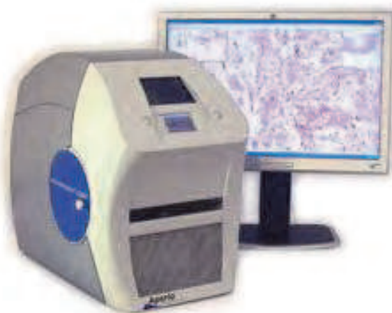
Fig. 11. For dynamic telepathology a slide scanner and a fast web connection with a server are mandatory. Costs are high but diagnostic and educational potentials are huge.
