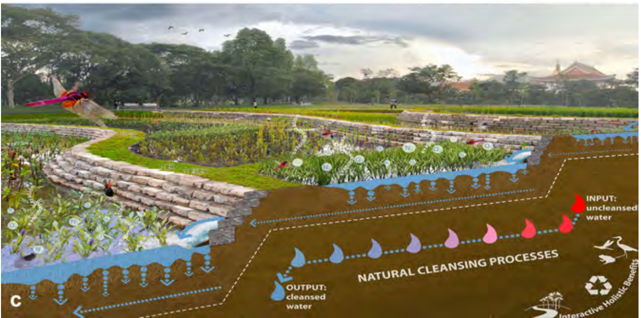
(Fig. 3) Bishan-Ang Mo Kio Park , Singapore. Project by Ramboll Studio Dreiseitl. 3a. The project area before and after interventions; 3b. Different river habitats along the project area; 3c. Technic-functional process diagram of the river terracing. Source: Atelier Dreiseitl.
