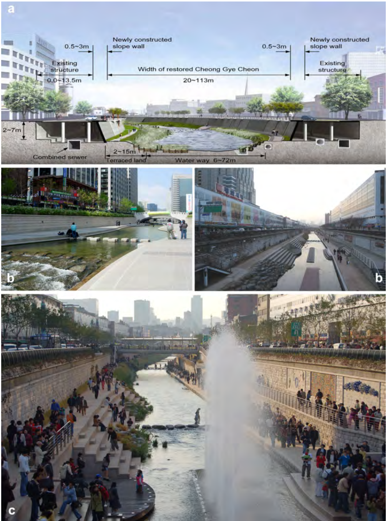
(Fig. 8) Cheong Gye Che , Seoul. Project by Cheongsuk Eng., Saman Eng. e Dongmyung Eng. + SeoAhn Total Landscape. 8a. Cross-section of the river restoration project; 8b; The restored riverbed between building and infrastructural pre-existences; 8c. A new co-evolutive season for the story of Cheong Gye Che river.
