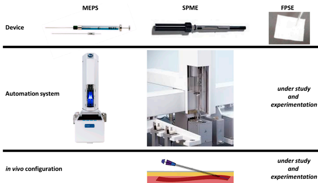
Figure 2. Current developmental stages and future perspectives of MEPS (micro-extraction on packed sorbent), SPME (solid phase microextraction), and FPSE (fabric phase sorptive extraction).
