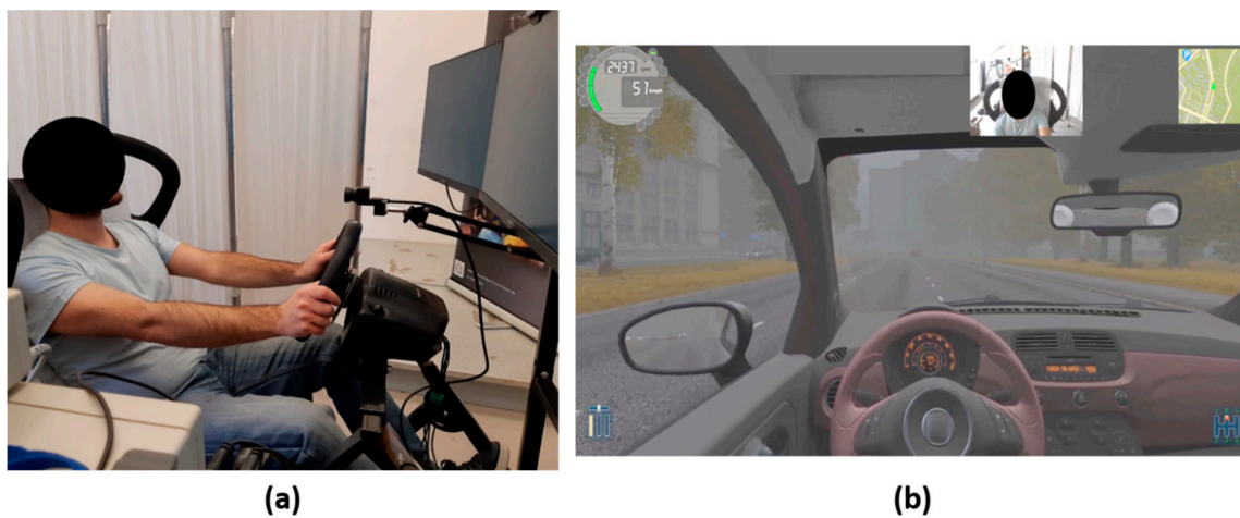
Figure 1. Experimental setting for the proposed study: (a) driving simulator, lateral view; (b) screenshot of the software used for the driving simulation: City Car Driving [34].
