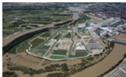
Figure 9: The 2008 floods highlighted the dual character of the park: behind the dike, the protected part with canals and pools; in front of the dike, the inundated, tree-covered flood plain. Photo by Hadajover.
