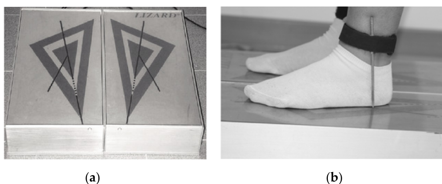
Figure 2. (a) Posture-stabilometric vertical force platform (Lizard; Lemax s.r.l., Como, Italy); (b) a custom tool for correct positioning of the subject on the platform.
