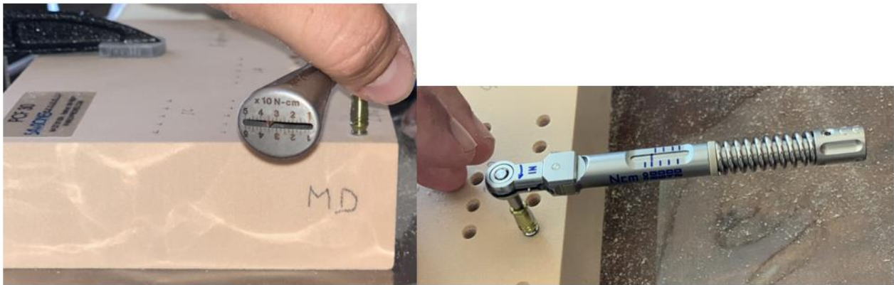
Figure 3. Details of the insertion and removal torque measured by the dedicated dynamometric ratchet.
