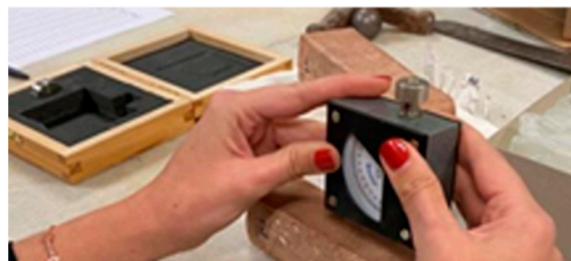
Figure 3. Measurement of surface hardness using the Shore D test on Geo_CBW samples.
