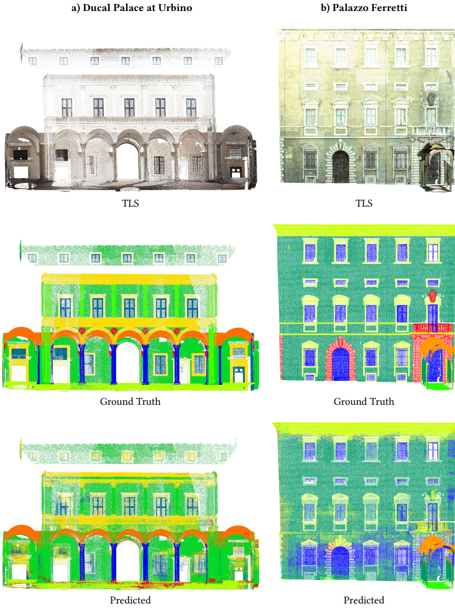
Fig. 7. Visualization of the result of the automatic segmentation of Ducal Palace at Urbino (a) and Palazzo Ferretti (b).
