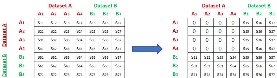
FIG. 19. Transformation of a similarity matrix into a forced similarity matrix. Two toy datasets has been used to show the forcing procedure. A which has 4 records and B which has 3 records. In this case, dataset A is forced to connect to dataset B .
