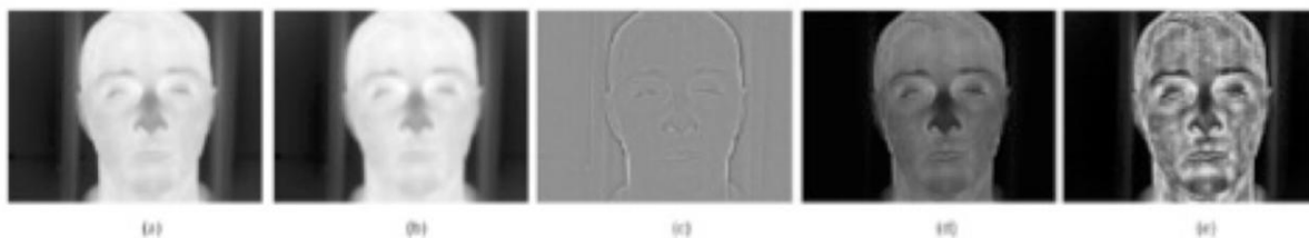
Fig. (A.1) - Thermal image enhancement. (a) Original thermal image, grayscale; (b) filtered image; (c) difference image [(a)-(b)]; (d) contrast enhanced image; (e) contrast-limited adaptive histogram equalization (CLAHE) of image.
