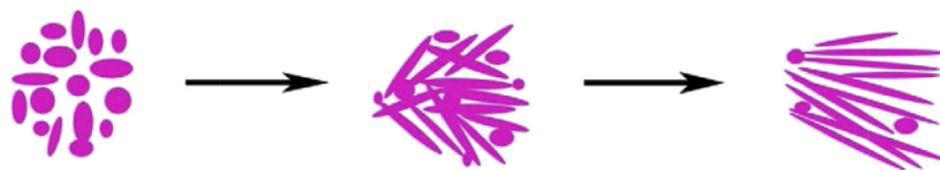
Scheme 23. Schematic representation of \text{NiMoO}_4 nanorods synthesized under silent conditions (left), US irradiation at 45 W (center), 75 W power (right) (Image reproduced from reference 98, by kind permission of Elsevier).
