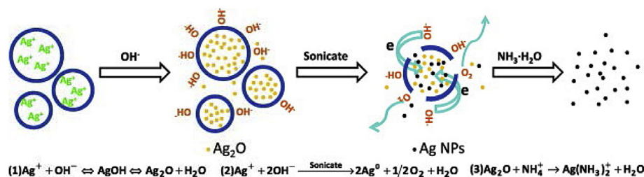
Scheme 25. Formation of Ag NPs in alkaline aqueous solution via US irradiation (Image reproduced from reference 106, by kind permission of Elsevier).
